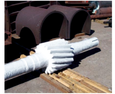
Above: A large Enviropeel-protected component is in stark contrast to the unprotected steel in the background.
